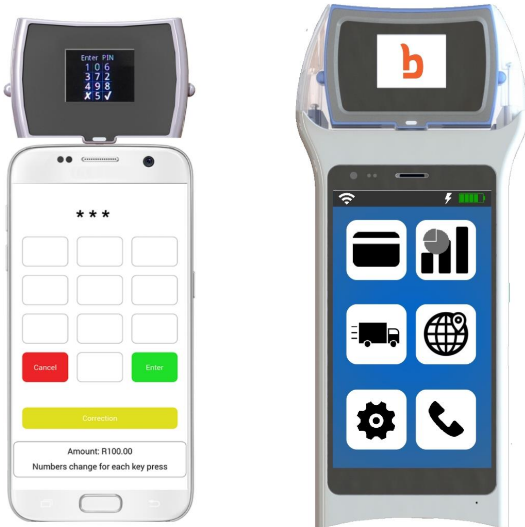
Figure 1 : Payment Pebble® version tCR2 as a bring-your-own-device solution (left), and as part of the Thumbzup Payment Blade (right)
